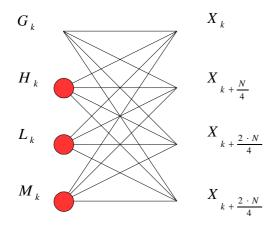
This butterfly requires 3 complex multiplications:  $W_N$  matrix can be calculated without any multiplication. Applying this butterfly to a 4-samples sequence yields:  $G_K = \{x_0\}, H_K = \{x_1\}, L_K = \{x_2\}, M_K = \{x_3\}$  and:
