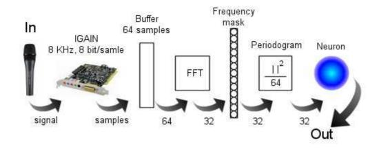
The signal is read from the internal PC's microphone, pre-amplified according to SoundBlaster's input gain (IGAIN), sampled by the SoundBlaster's DSP and saved into a 64-samples buffer.
